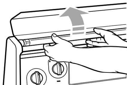
5. Replace tube, replace top of the control panel.
