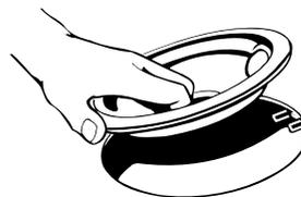
2. Holding the coil element as level as possible, carefully push coil element terminal into the receptacle.
